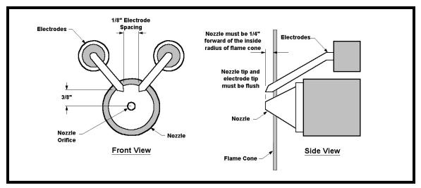
Figure 37 – Electrode Adjusment Diagram
